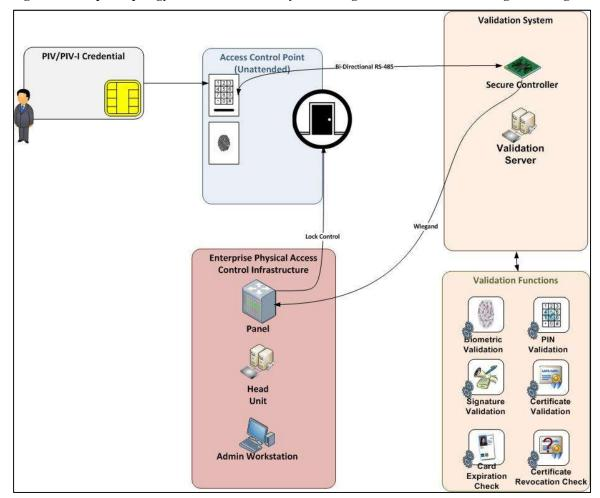
Figure 1 - Sample Topology for an End-to-End System Using FIPS 201 Evaluation Program Categories
